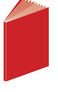
PUR binding is the same method as perfect binding, but uses a different adhesive. PUR (polyurethane reactive) glue holds stronger than standard perfect binding glue and remains strong at temperature extremes.
