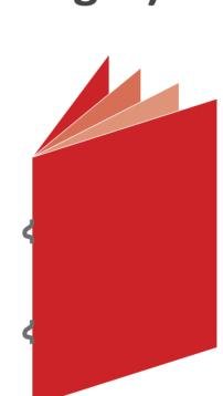
Comparable to saddle stitching, but with a different effect. Loops are created with wire along the external spine in order to insert and secure the document into a 3-ring binder. Great option for information installments that can be added to larger collection.
