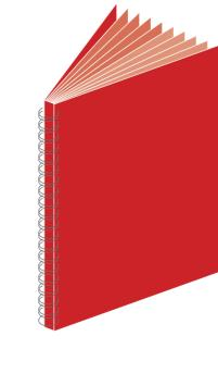
Highly popular Wire-O option uses formed wire that threads through punched holes. This allows books to lay flat when open. Wire loops are available in variety of colours to coordinate with cover colour. A durable option for a wide variety of project.
